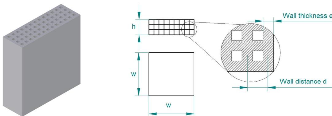
**Picture 3:** Test specimen manufactured with LMF
