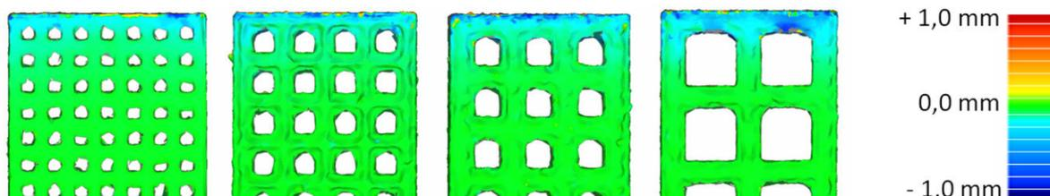
**Picture 5:** Geometric deviation of LMF substrate after LMD welding, determined by 3D scan
