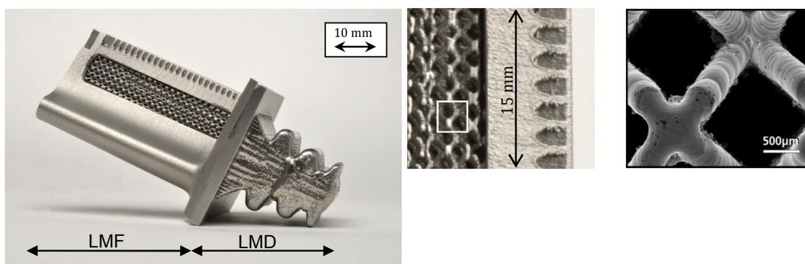
**Picture 6:** Turbine blade manufactured by LMF and LMD
