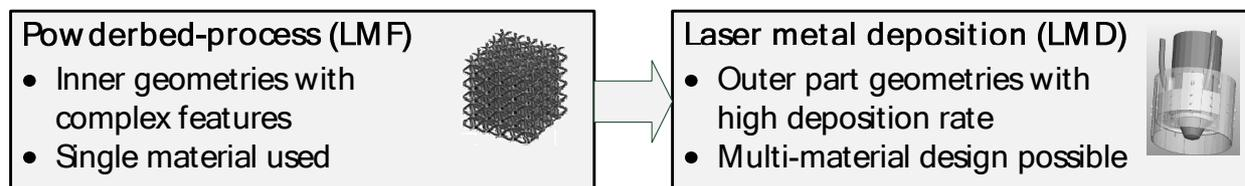
**Picture 2:** Combined additive manufacturing
