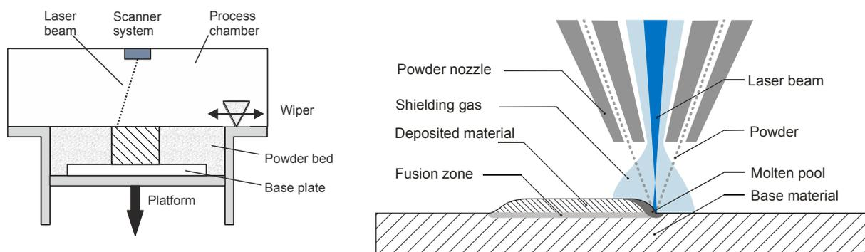
**Picture 1:** (a) Laser metal fusion process; (b) Laser metal deposition process
