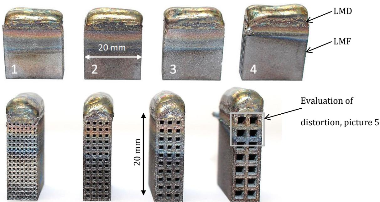
**Picture 4:** Heat tint on test specimen after LMD deposition
