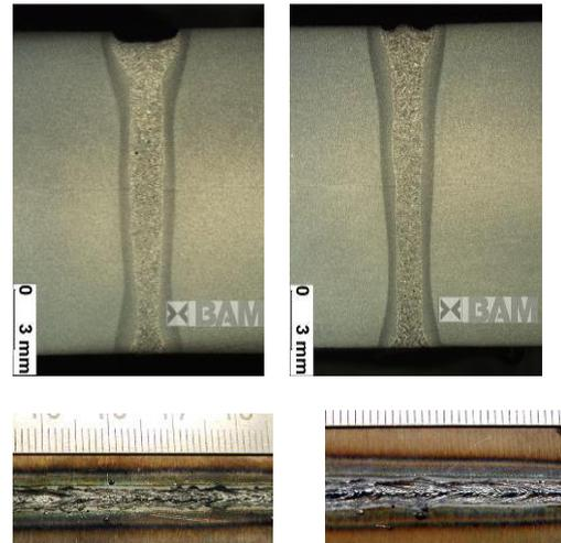
**Fig. 7:** Positional welding PF (up) 90°,
