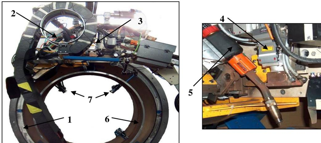
Fig. 2: Orbital welding device with welding head
