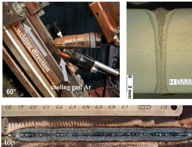
**Fig. 6:** Positional welding PF (up) 60°,
