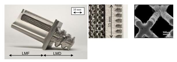
Picture 6: Turbine blade manufactured by LMF and LMD
