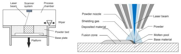
**Picture 1:** (a) Laser metal fusion process;
