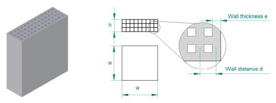
Picture 3: Test specimen manufactured with LMF
