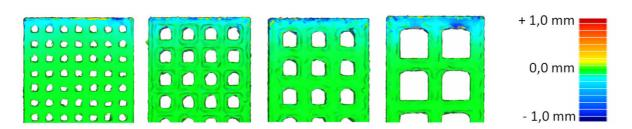
Picture 5: Geometric deviation of LMF substrate after LMD welding, determined by 3D scan
