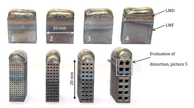
Picture 4: Heat tint on test specimen after LMD deposition
