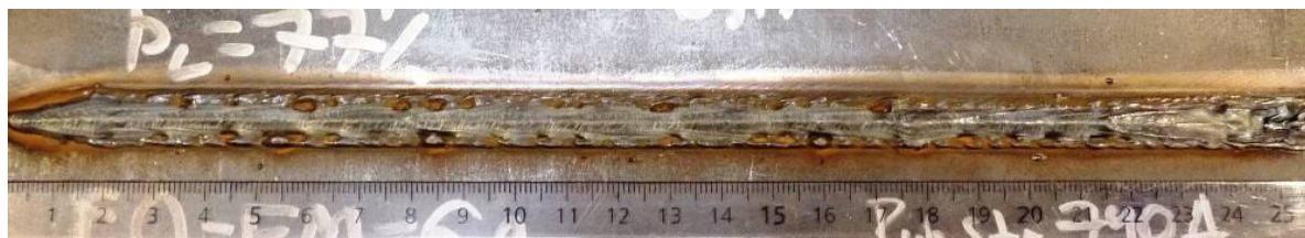
Fig. 4: Laser hybrid welding with modified spray arc, undercuts
