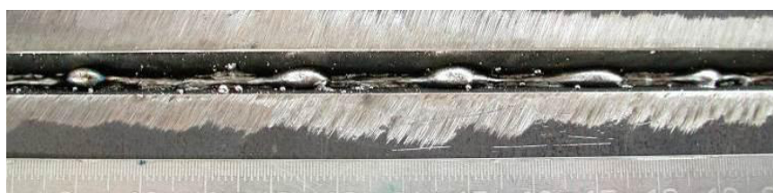
Fig. 5: Laser hybrid welding with modified spray arc, excessive penetration
